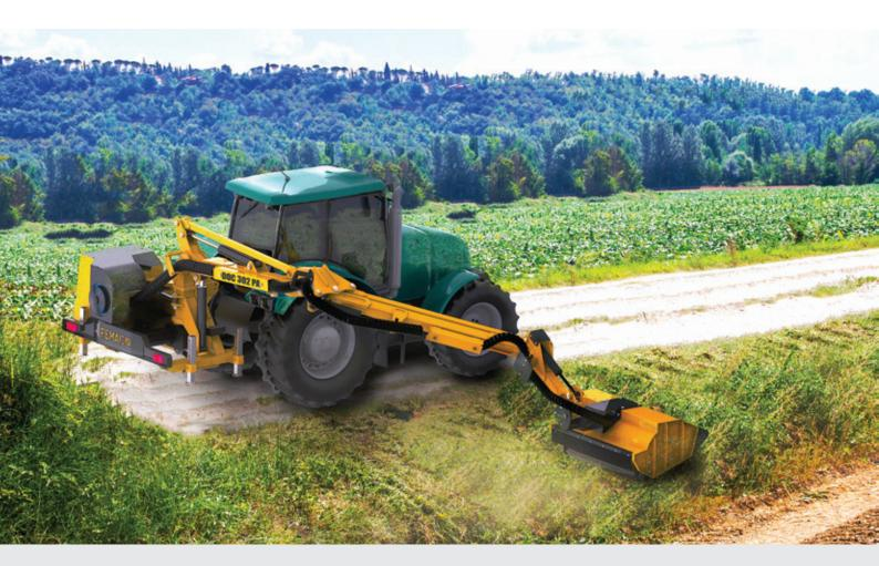
Hydraulic hedge mower with the side cabin forwarding and 100° rotating column with shock resistant hydraulic safety device for tractors HP 100/130 and weight 3500/4500 kg, suitable for working on local and trunk roads and farms.
