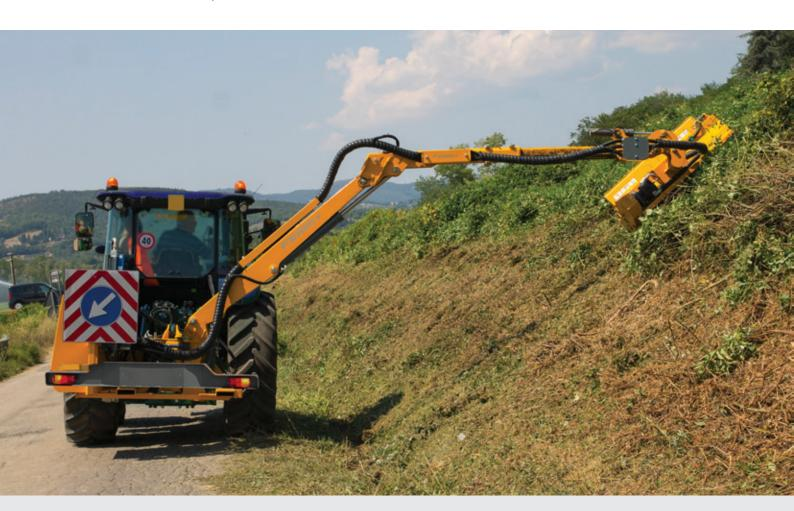
Hydraulic hedge mower of 7.5 m range, for tractors HP 130/180 and weight 6500 kg, suitable for heavy drainage and road mowing, strong, compact, connected on the tractor in high position and fast on the motions.
