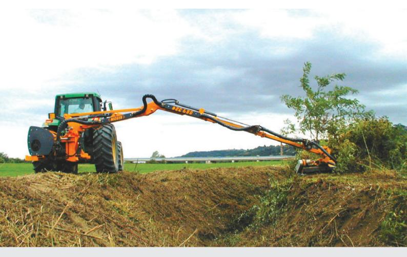
Hydraulic hedge mower of 9 m range, for tractors HP 150/200 and weight 7000 kg, suitable for heavy drainage and road mowing, strong, compact, connected on the tractor in high position and fast moving.
